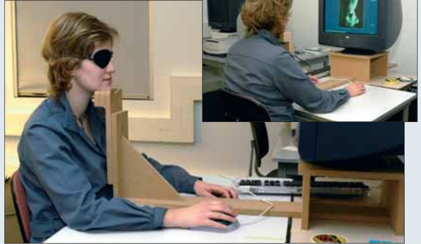
View showing a subject (in this case, doctorate student Els Cornelis) using the test set-up. To ensure a constant viewing distance, a chin rest is used. The eye patch is to ensure that the test subject uses only one eye to view the scene. The markers are adjusted using a computer mouse.
