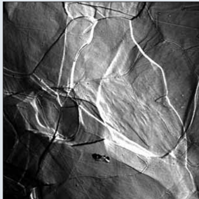
Microscope view of austenite in pure iron. The image was obtained using a laser-scanning confocal microscope at a temperature of 1000 °C.
