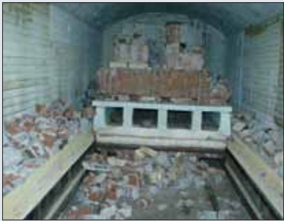
In three hours, the rubble was heated to a temperature of 540 °C. After two hours at that temperature, the cooling stage followed. The bricks, which had been stacked high inside the kiln, had broken apart from the mortar and tumbled from the kiln lorry.
