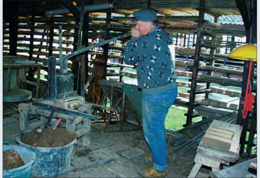
At the Kijfwaard brickworks at Pannerden, a test was conducted in which the brick fraction, after being ground, was mixed with clay in a 50/50 mix. Using the common Dutch production method with moulds (because of the soft clay), the mixture can be used to produce bricks. The clay mass is pressed into moulds that have been sanded to make the unfired bricks easier to extract.
